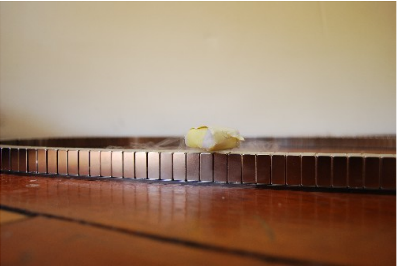
Figure 10: Superconductor levitating above the oval track.
