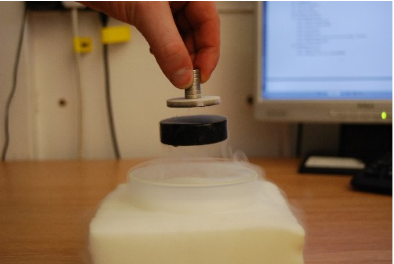
Figure 6: Superconductor raised up with magnet.
