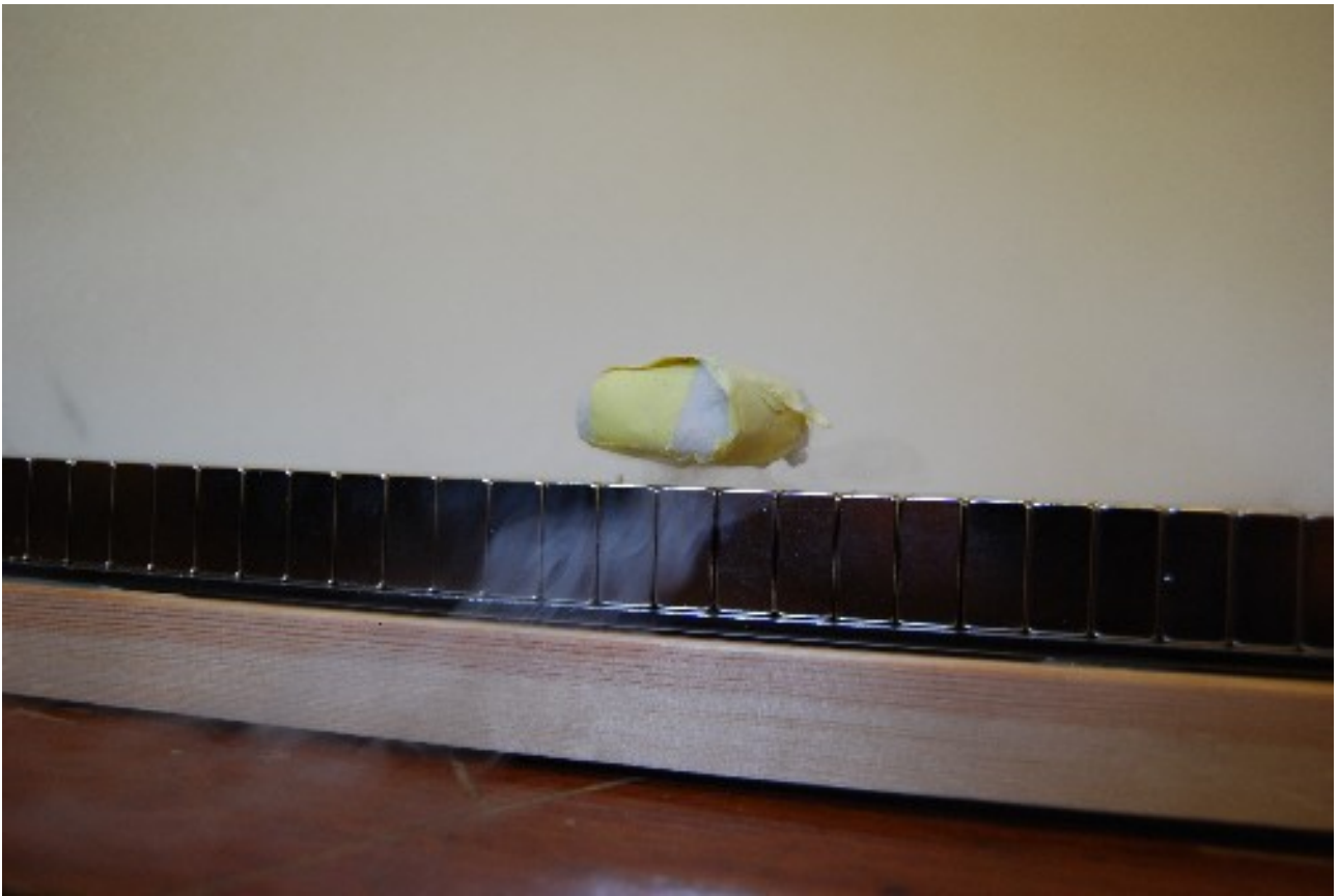
Figure 9: Superconductor levitating above a linear track.
