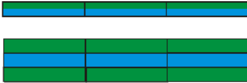
Figure 7: Configuration of magnets for a magnetic track. Green is north and blue is south. Top is side view at edge of track and bottom is top view.
