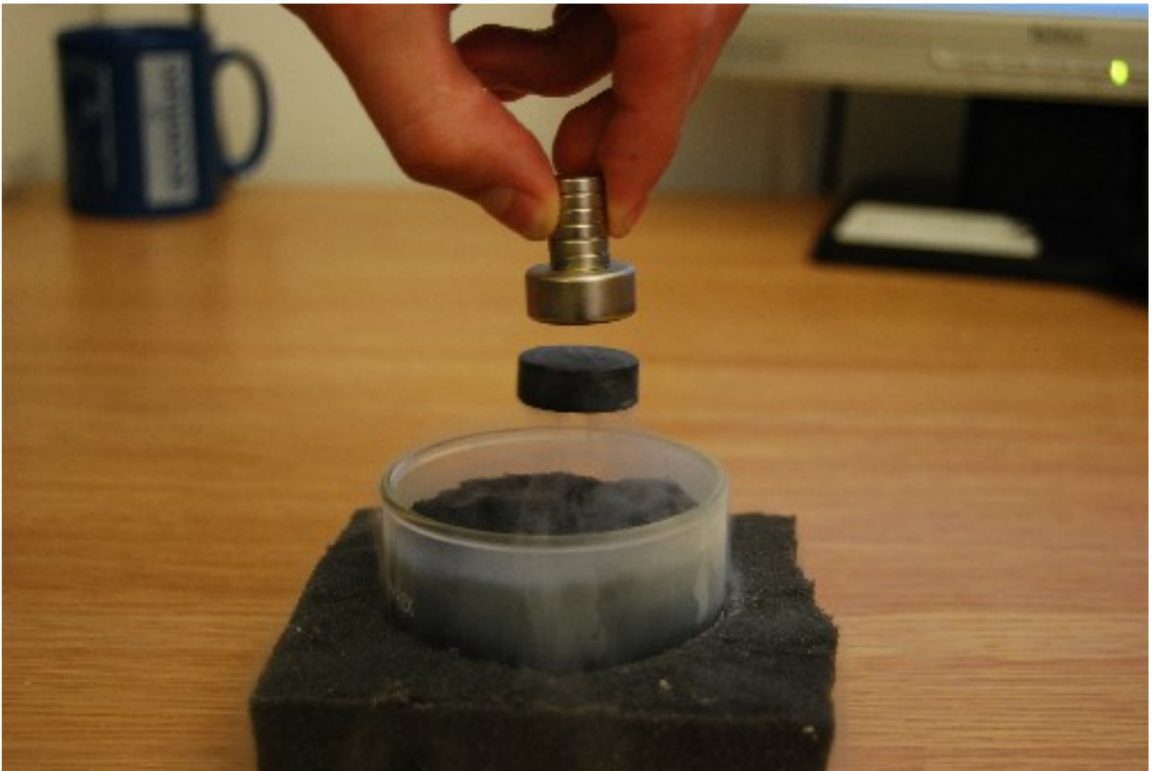
Figure 3: Superconductor raised up with magnet
