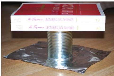
**Figure 3.** Phone in the tin, with a textbook to ensure there are no unwanted gaps in the Faraday cage.
