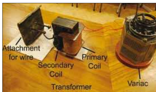
Figure 1. A diagram of the equipment, which shows the Variac (right) that is connected to the transformer (middle) and the coat-hanger wire (left). The coat-hanger wire is attached through a shield made from a heat-proof mat and is placed on a heat-proof mat. Safety screens should be in place when this equipment is used to protect both the pupils and the teacher.
