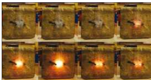
Figure 2. Composite image showing eight frames in succession of the thick coat-hanger wire as it melts due to the heat generated by the high current passing through it.
