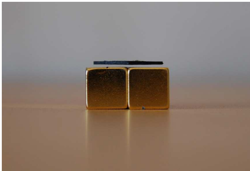
Figure 2. Photograph showing a piece of pyrolytic graphite levitating above permanent magnets.
