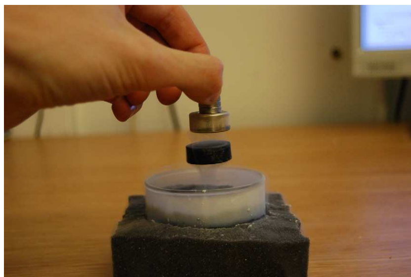
Figure 5. Superconducting levitation demonstration using a neodymium magnet (silver) and a superconductor levitation disc (black).
